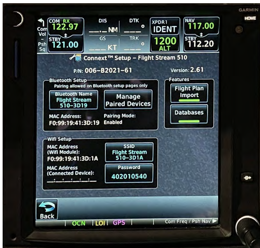
Garmin GTN 750/650 setup. Under Bluetooth Setup, tap Manage Paired Devices.
